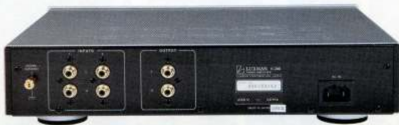
ABOVE: Luxman provides for two MM or MC pick-ups to be connected at once
